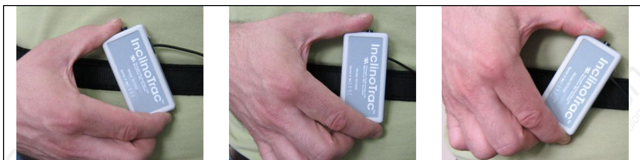
Twist the inclinometer sideways two or three times while holding it firmly against the strap
